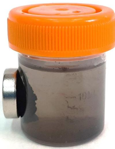
AC- $\text{Fe}(\text{NO}_3)_3$  activated carbon has very strong magnetic properties.
