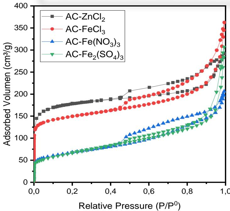
Micro-mesoporous character of activated carbons: N<sub>2</sub> adsorption-desorption isotherms Type IV, according to IUPAC classification
