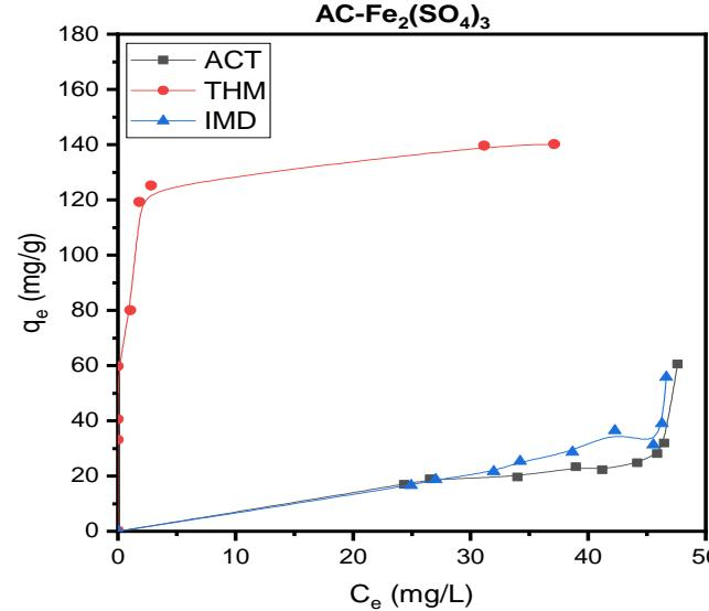
Adsorption isotherms type **S3** and **S4**, according to Giles and col. classification
